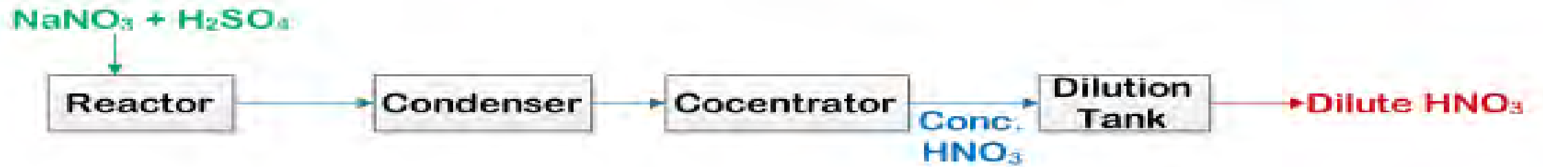
Figure: Manufacture of nitric acid from chile saltpetre or nitrate
