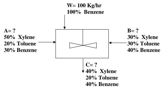
Solution: By making component material balance on each component within the mixer you can reach to a system of three equations which can be solve by using the command solve to find the unknowns A, B, C.
