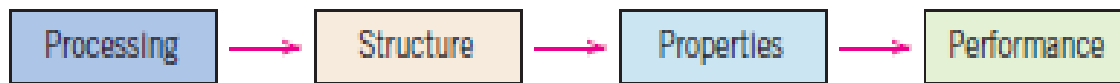
Figure 1.1 The four components of the discipline of materials science and engineering and their interrelationship.
