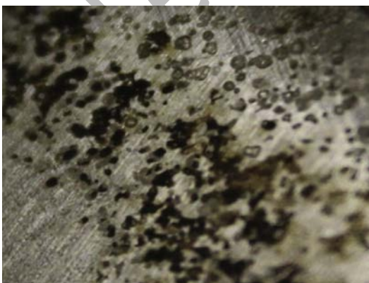
Pits on 304 stainless steel after exposure to simulated marine environment
