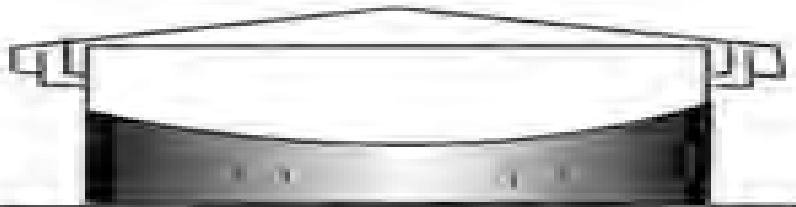
LIFTER ROOF TANK
