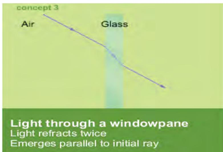
Wavelength of light in different media When light changes speed as it moves from one medium to another, its frequency stays the same but its wavelength changes. The
