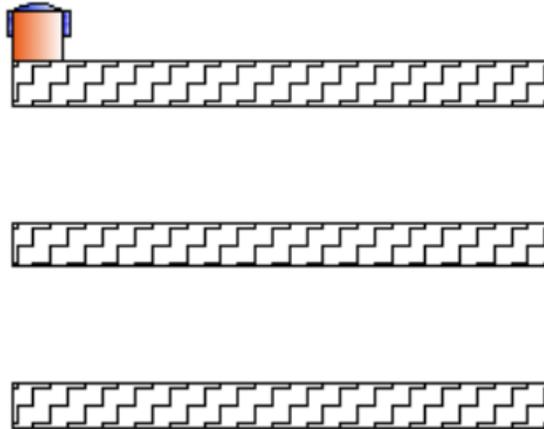
In this example, we will create a matrix of the element shown in the drawing, with 3 lines and 5 columns, and since we want the rows below the element, we will enter a value of 30 and for the columns 20, because we want to repeat the columns to the right.
