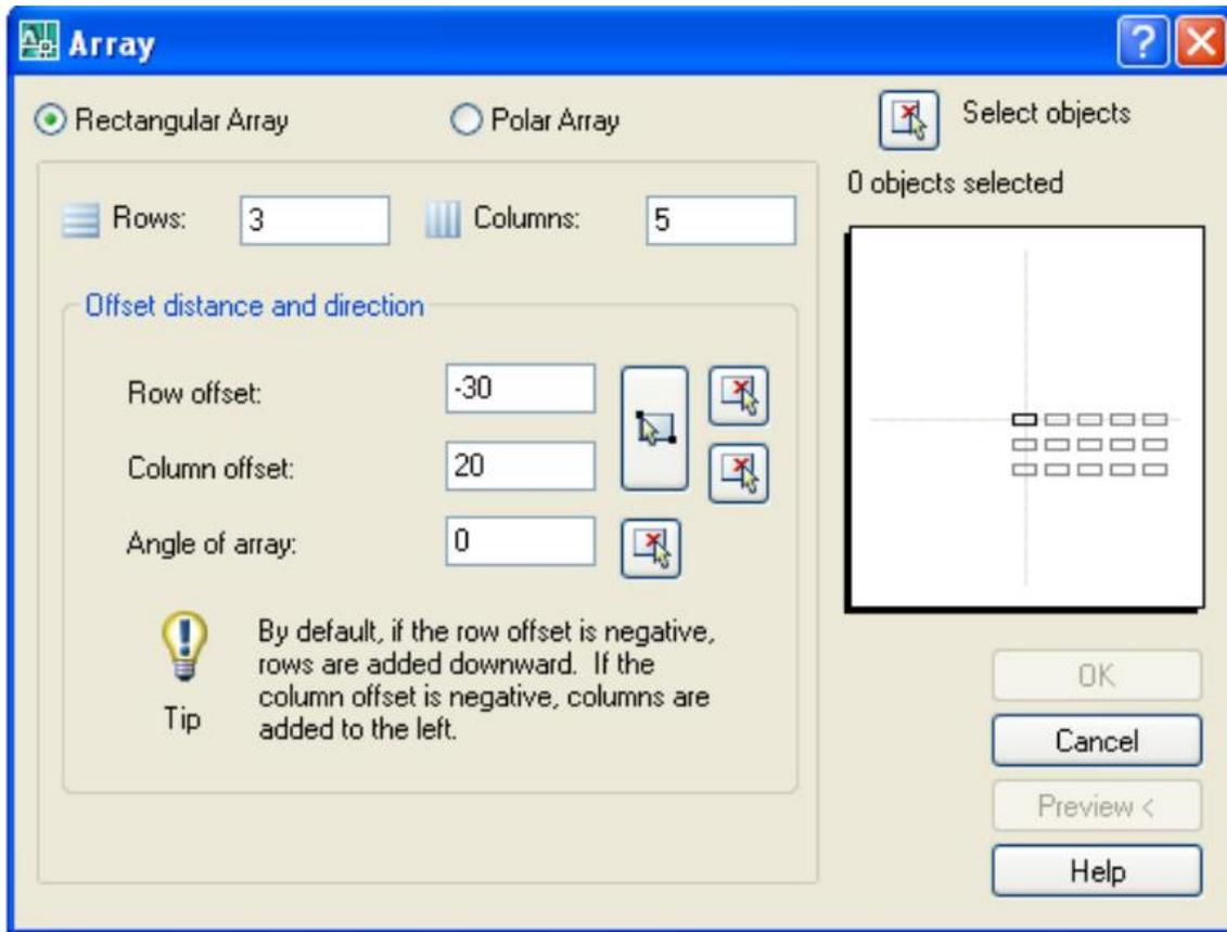
Now select the element to be repeated by pressing the **Select object** button on the
