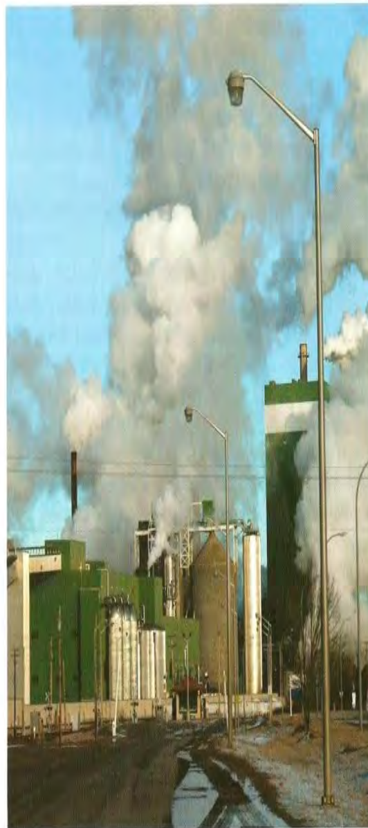
Figure 16.7 The most annoying pollutants from this paper mill are pungent organosulfur thiols and sulfides. Chlorine bleaching can also produce extremely dangerous organochlorines, such as dioxins.
