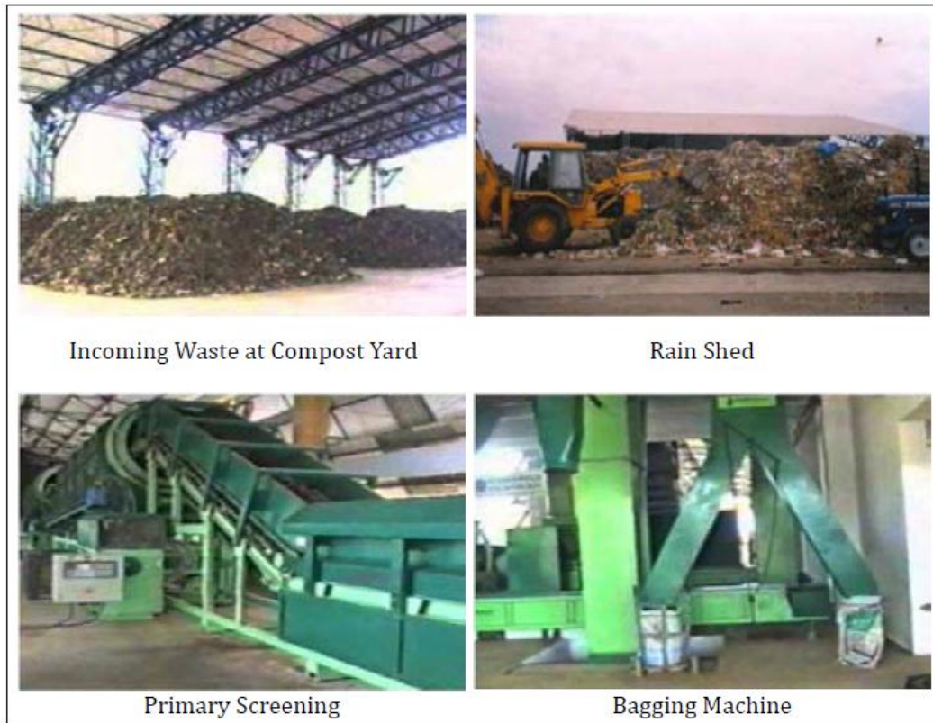
Figure 3.16: Unit operations in windrow composting
